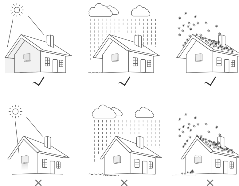
▲ Figure 4.1 Recommended Installation locations
